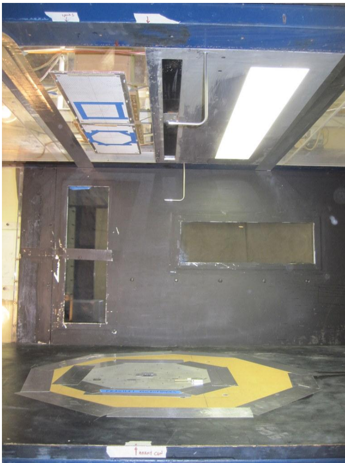
Figure 1. Test setup in the wind tunnel test section with phased array in the bottom, speakers in the top, and two pitot static tubes attached to the ceiling. A hot-wire probe for boundary layer measurements is retracted to the surface of the array plate. The flow moves from left to right.
