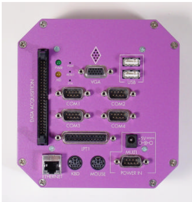
Front panel showing 14 screwlocks installed into 7 Dsub connectors
