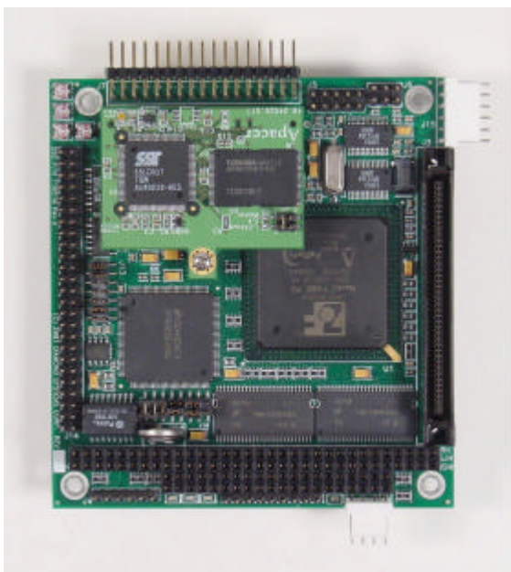
Flashdisk mounted onto CPU
