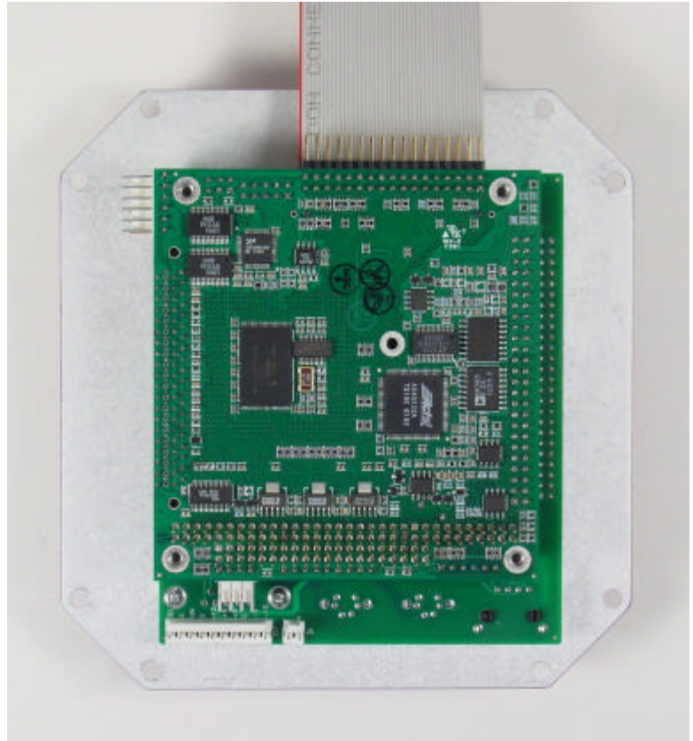
CPU with IDE cable mounted on stack
