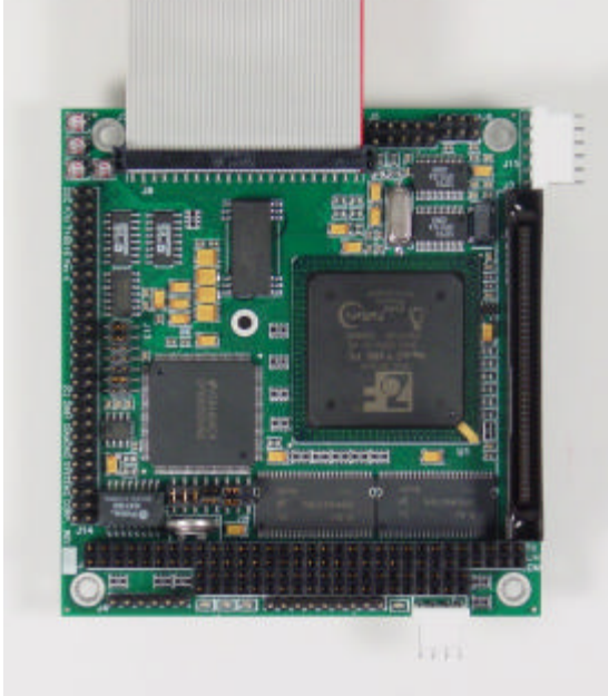
CPU with IDE cable installed
