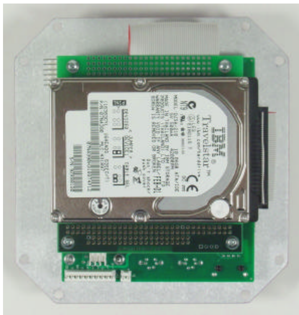
Hard drive mounted onto stack
