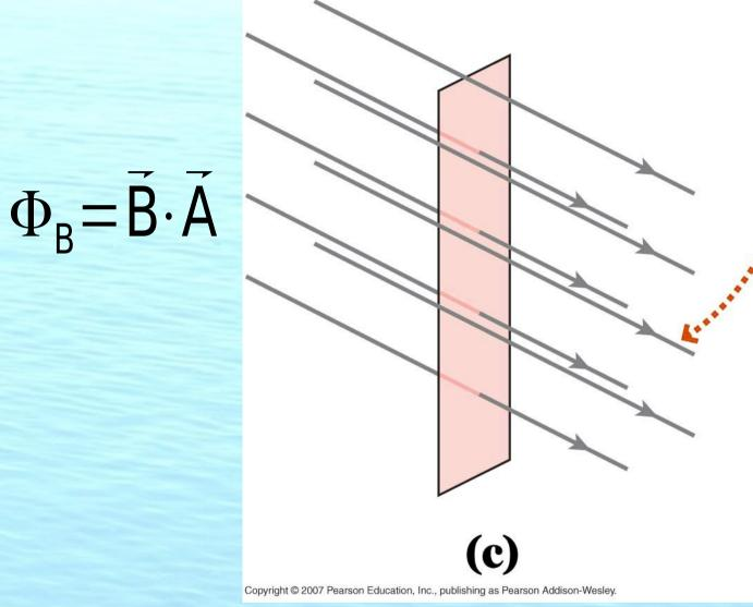
A smaller surface area than in (b) reduces the flux.
