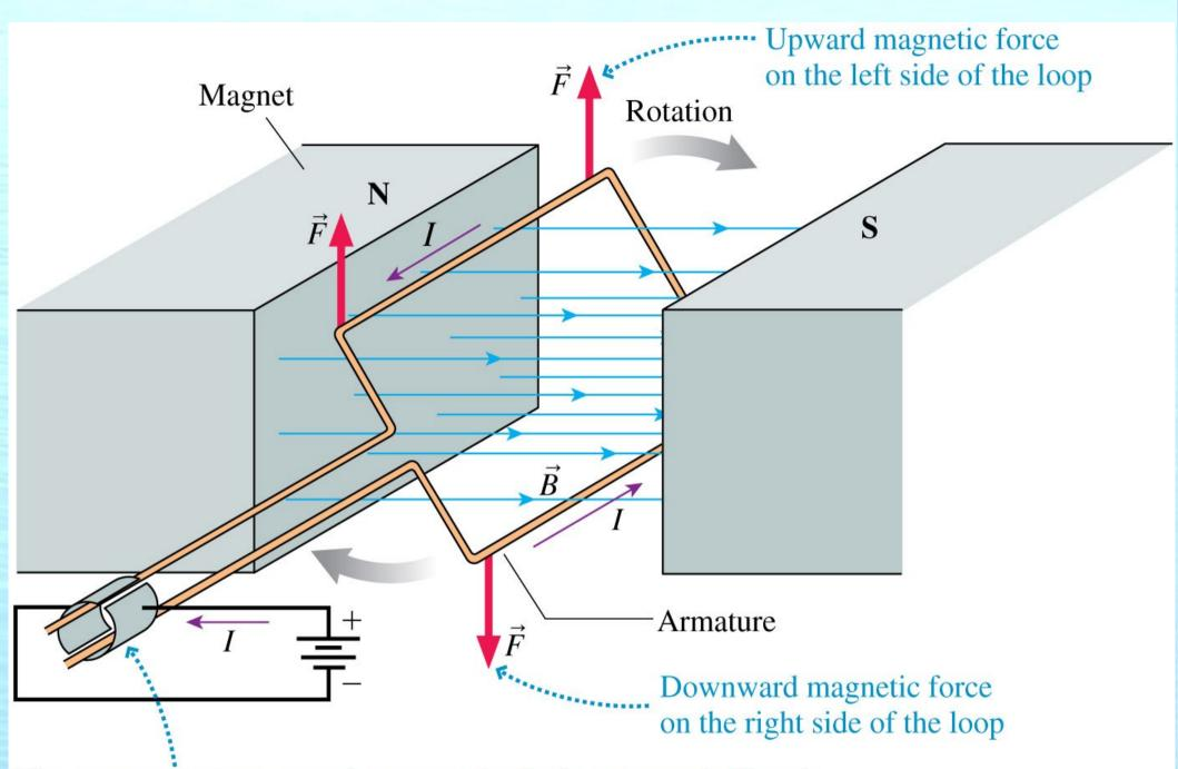
The commutator reverses the current in the loop every half cycle so that the force is always upward on the left side of the loop.
