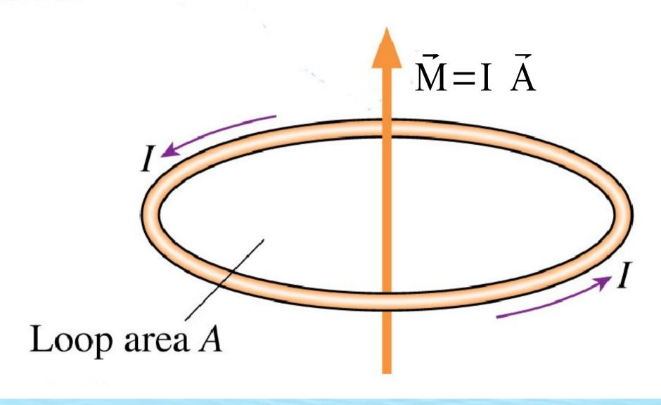
Torque on a current loop is proportional to magnetic moment.
