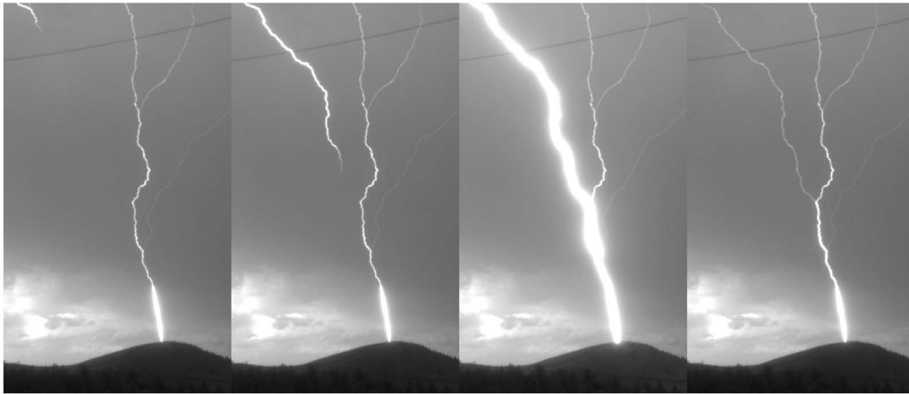
Figure 5. Camera frames beginning at 0.905625 s after 20:42:09 UTC showing a dart leader traveling down the dark branch 1, merging with the luminous branch 2, and initiating a return stroke upon reaching the ground. The exposure time for each frame is 150 \mu\text{s} . The time interval from the beginning of one frame to the beginning of the next frame is 156 \mu\text{s} except for the last frame, which follows the beginning of the third frame by 469 \mu\text{s} . The vertical distance from the triggering site to the altitude at the top of the frame is about 1 km.
