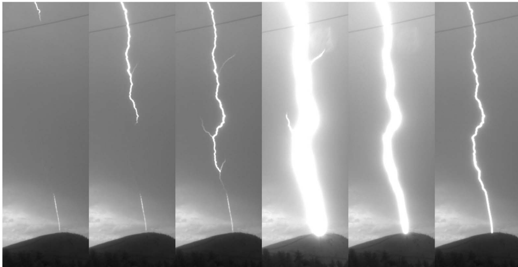
Figure 6. Consecutive frames beginning at 1.209842 s after 20:42:09 UTC showing a dart leader traveling down branch 2. The dart leader initiates luminous waves that travel up the branches it meets and is followed by a reflection (return stroke) upon reaching the ground. The return stroke also initiates luminous waves upward along branches at junctions, just like the dart leader did. The exposure time for each frame is 150 \mu\text{s} . The time interval from the beginning of one frame to the beginning of the next frame is 156 \mu\text{s} . The vertical distance from the triggering site to the altitude at the top of the frame is about 1 km.
