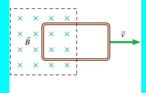
**Problem 7:** A single-turn rectangular wire loop has a resistance equal to 1.4 M and the dimensions shown in the drawing. The magnetic field at all points inside the loop varies according to  $B=B_0e^{-\alpha t}$ , where  $B_0=0.25$  T and  $\alpha=200~{\rm s}^{-1}$ .
