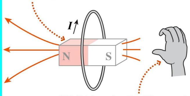
Right-hand rule: Fingers in direction of current point thumb in direction of N pole.
