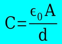
[Ex. 1] Find the capacitance of a parallel plate capacitor consisting of circular plates 10 cm in radius separated by 1.5 mm.
