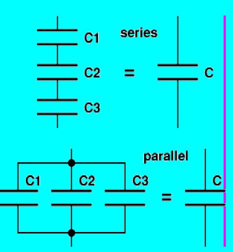
Caps in series have the "bottom wire" or one Connected to the "top wire" Of the next.
