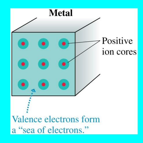
• The solid as a whole remains electrically neutral, but the electrons are now like a negatively charged liquid permeating an array of positively charged ion cores. You rub a teflon with rabbits fur and make it negatively charged.
