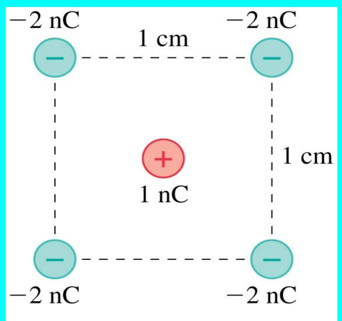
Estimate the direction and magnitude of the NET force on the central charge due to the other four charges.
