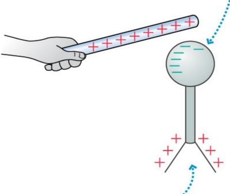
Although the net charge on the electroscope is still zero, the leaves have excess positive charge and repel each other.
