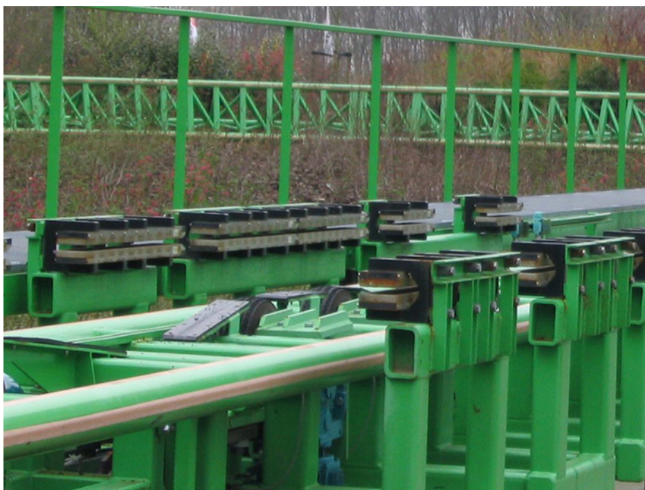
Figure 13.26 The rows of rare-earth magnets (protruding horizontally) are used for magnetic braking in roller coasters. (credit: Stefan Scheer)
