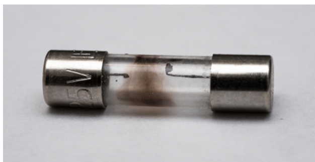
Figure 9.25 A fuse consists of a piece of wire between two contacts. When a current passes through the wire that is greater than the rated current, the wire melts, breaking the connection. Pictured is a “blown” fuse where the wire broke protecting a circuit (credit: modification of work by “Shardayyy”/Flickr).
