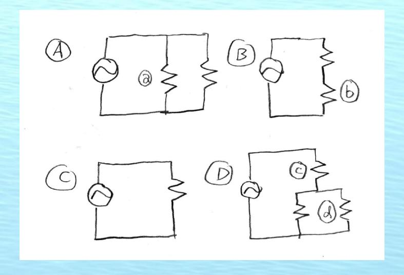
All of the resistors have the same value. Each of the power supplies is a constant voltage supply (and all are equal). Which circuit uses the *least* power?
