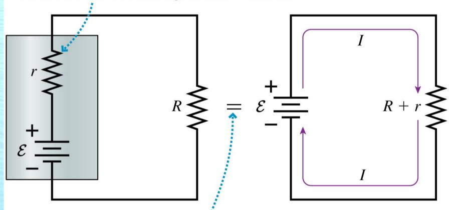
This means the two circuits are equivalent.
