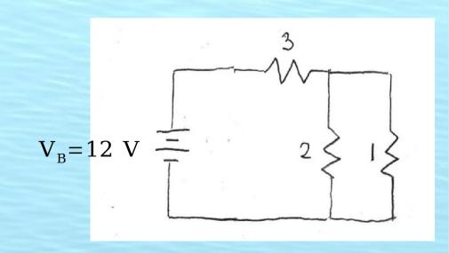
All of the resistors have the same value. Each of the power supplies is a constant voltage supply (and all are equal). Which circuit uses the most power?
