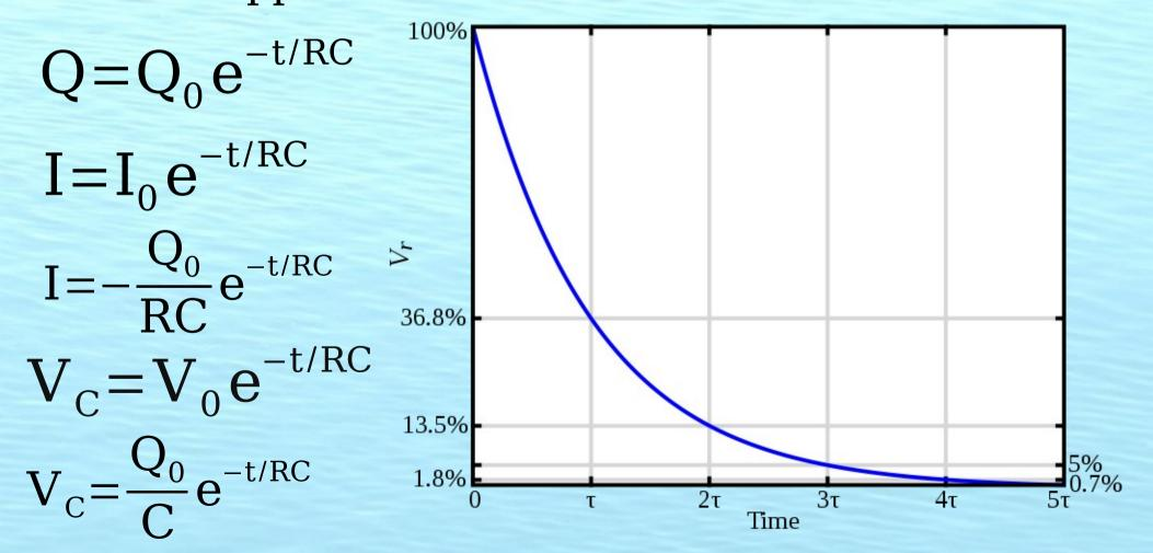
A 200 k $\Omega$  resistor is in series with C=10  $\mu$ F. A t=0, the voltage on the capacitor is 8 V. What is the voltage on the capacitor and the current through the resistor after 1 sec, 2 sec and 4 seconds?
