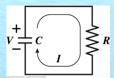
A 200 k $\Omega$  resistor is in series with C=10  $\mu$ F. A t=0, the voltage on the capacitor is 8 V. What is the voltage on the capacitor and the current through the resistor after 1 sec, 2 sec and 4 seconds?
