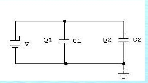
Two capacitors are connected together as shown. What is the equivalent capacitance of the two capacitors as a unit?
