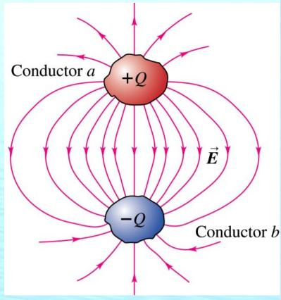
[Ex. 2] A capacitor's plates hold 1.3  $\mu$  C when it is charged to 80 V. What is its capacitance?
