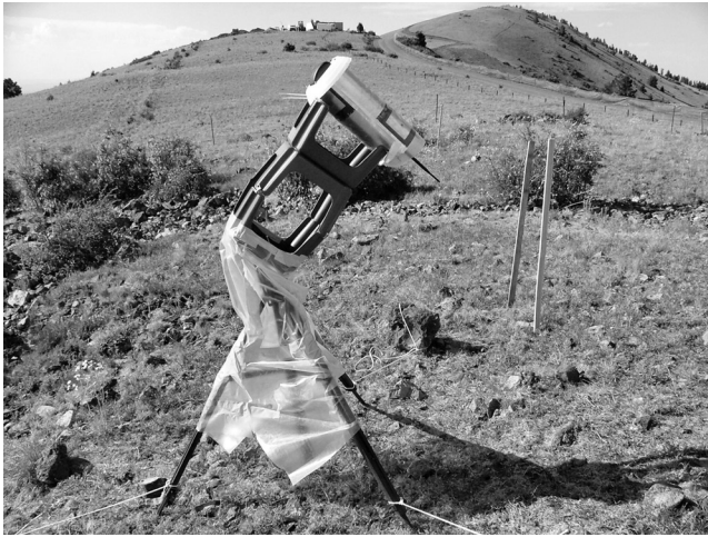
Figure 4. The Esonde calibration stand is made of a dielectric material which holds the Esonde 2 m above the ground with the vertical axis inclined by roughly 45^\circ .
