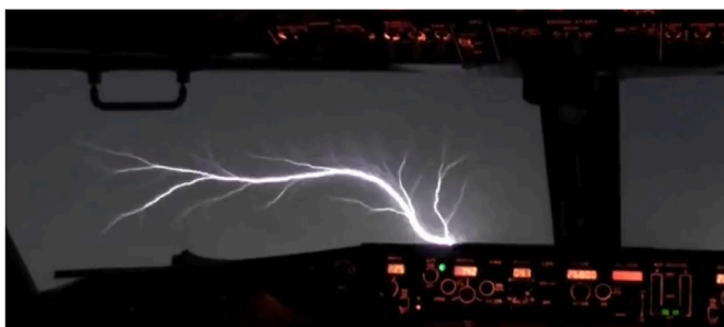
Fig. 5. Discharges from the windshield of a Boeing 737NG to the fuselage, repeating with a period of about 3 s. From YouTube/PilotsTubeHD, with permission.
