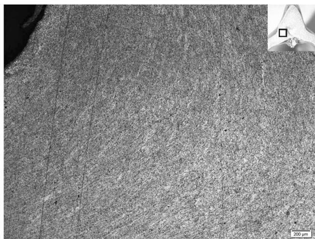
**Figure 17.**  $50\times$  optical microscopy examination of aluminum liner.
