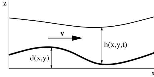
Figure 5.1: Definition sketch for derivation of the shallow water equations. The layer of water has thickness  $h$  which is a function of position and time. The flow velocity  $\mathbf{v}$  varies with position and time, but is assumed to be primarily horizontal and to not vary significantly with height. The terrain over which the water flows has elevation  $d$  which is a function of position. The sketch is two-dimensional, but we derive the full equations valid in three dimensions.
