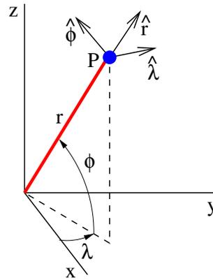
Figure 5.3: Spherical coordinate system used in this chapter. The longitude is  $\lambda$  and the latitude is  $\phi$ . A local Cartesian coordinate system is defined at point P with eastward, northward, and upward unit vectors defined as  $\hat{\lambda}$ ,  $\hat{\phi}$ , and  $\hat{r}$ .
