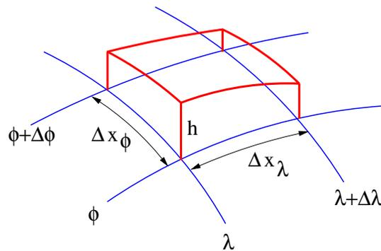
Figure 5.4: Sketch used to obtain shallow water mass continuity equation on a sphere.
