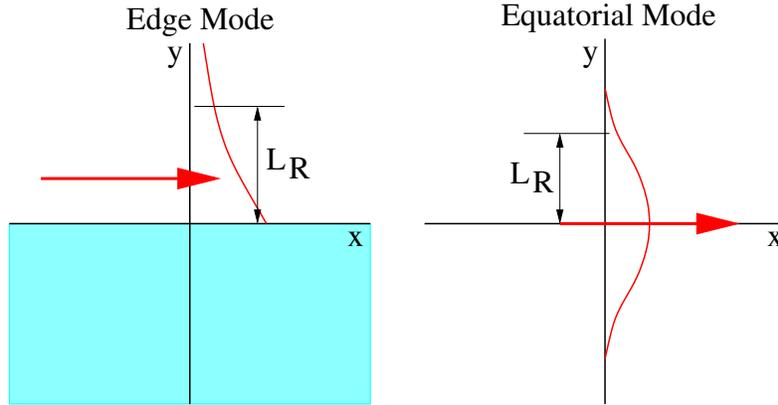
Figure 5.2: Two types of Kelvin wave moving in the  $+x$  direction, an edge wave (left) and an equatorial Kelvin wave (right). The transverse dimension of the wave scales with the Rossby radius  $L_R$ .
