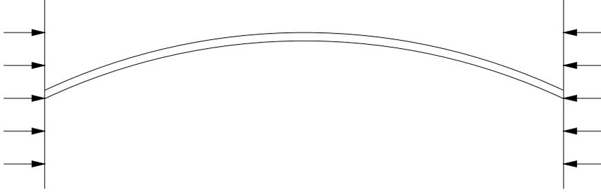
Figure 7.4. Buckling of a thin beam under compression.
