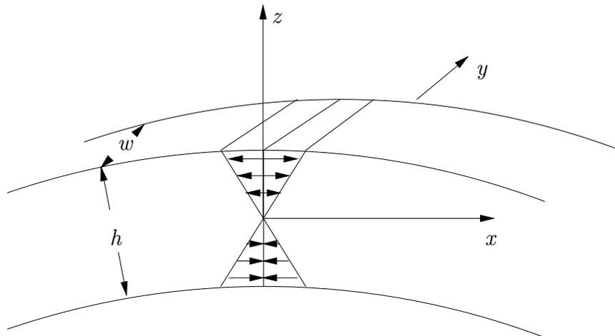
Figure 7.2. Section of a bent beam. The upper part of the beam is in tension, the lower part, compression.
