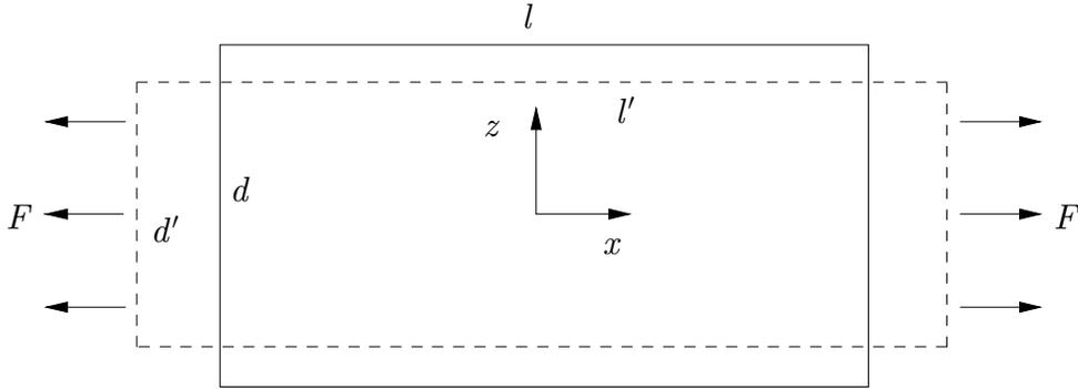
Figure 5.1. Deformation of a rectangular parallelepiped under the influence of uniform normal tractions on the left and right ends.
