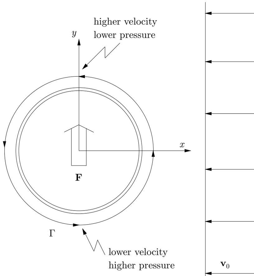
Figure 10.8. Lift acting on a rotating cylinder.
