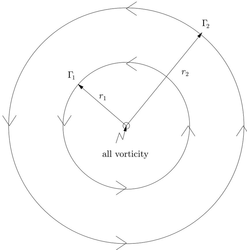
Figure 10.3. Two circulation loops around a point vortex. The circulations are equal, i. e.,  $\Gamma_1 = \Gamma_2$ .
