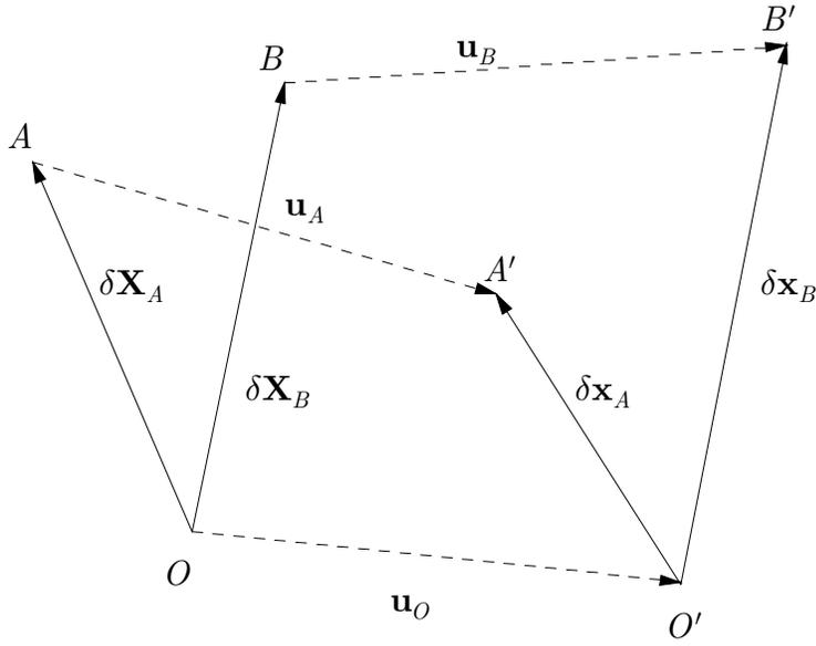
Figure 4.2. Displacement of three points,  $A$ ,  $B$ , and  $O$ .
