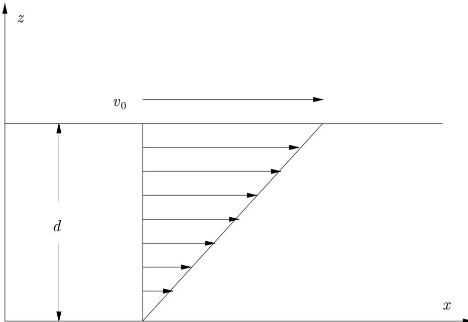
Figure 9.1. Creeping flow between two parallel plates, one of which is moving.
