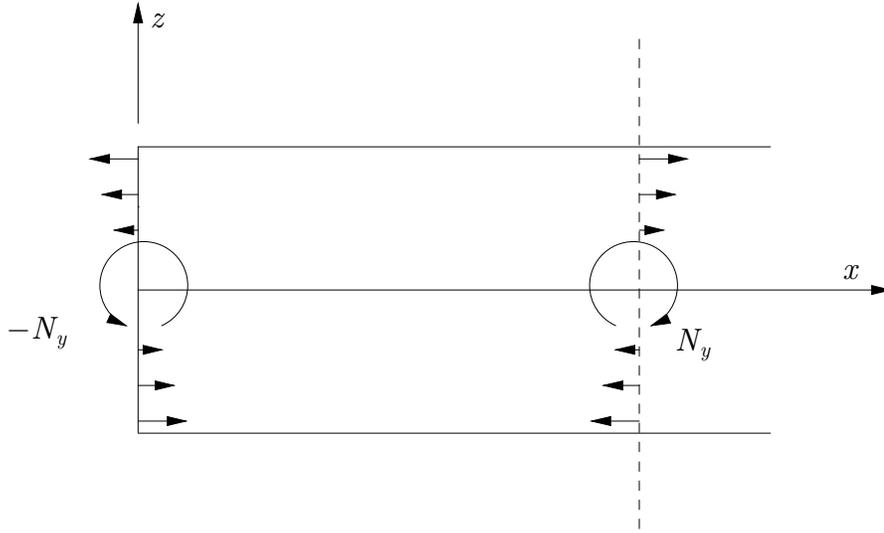
Figure 7.3. Tractions occurring at the ends and across a surface normal to a beam that is undergoing bending. The tractions result in a torque (or bending moment) in the  $y$  direction.
