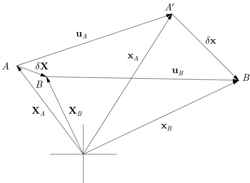
Figure 4.1. Relationship between the displacements of two parcels,  $A$  and  $B$ .
