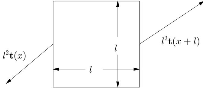
Figure 3.1. Definition sketch for computing the force imbalance on a cube. On the left side of the cube, the force is  $l^2 \mathbf{t}(x) = -l^2 [T_{xx}(x)\mathbf{i} + T_{xy}(x)\mathbf{j} + T_{xz}(x)\mathbf{k}]$ , while on the right side, it is  $l^2 \mathbf{t}(x+l) = l^2 [T_{xx}(x+l)\mathbf{i} + T_{xy}(x+l)\mathbf{j} + T_{xz}(x+l)\mathbf{k}]$ .
