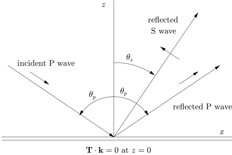
Figure 6.3. Illustration of the reflection of a P wave from a stress-free boundary at  $z = 0$ . Reflected P and S waves are created.
