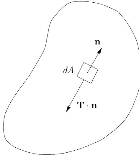
Figure 8.2. Illustration of the traction vector,  $\mathbf{T} \cdot \mathbf{n}$ , in a fluid at rest. This represents a normal compressional force on the fluid.
