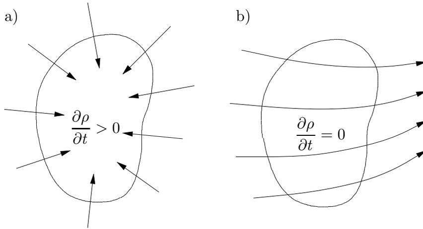
Figure 3.3. Illustration of a) divergent (actually, convergent) and b) nondivergent flow.
