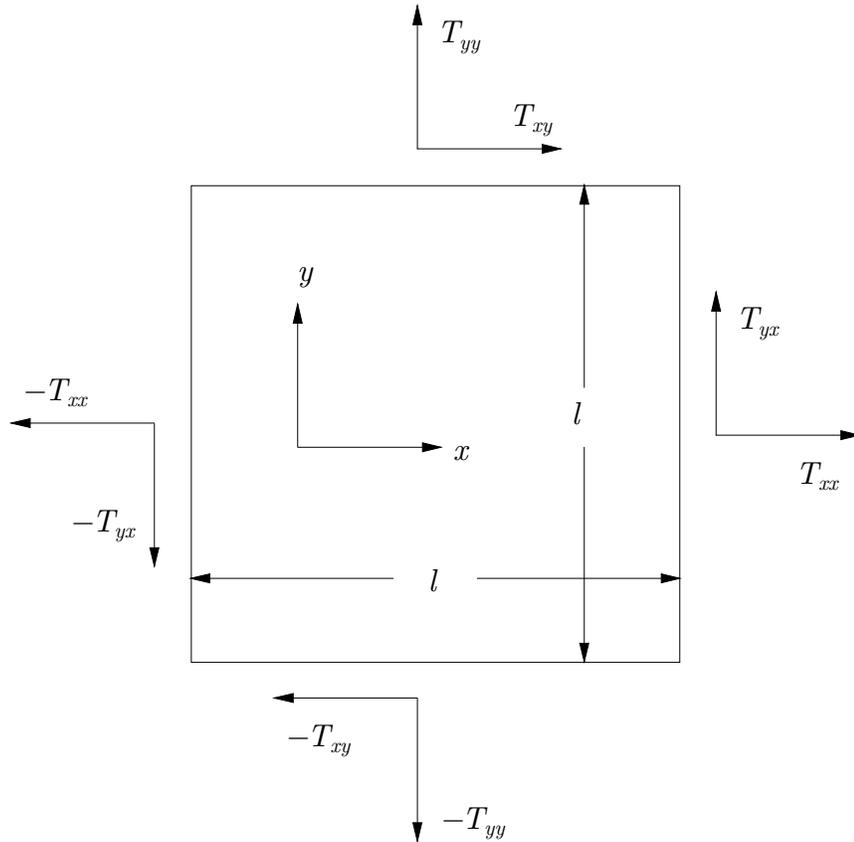
Figure 2.6. Illustration of stress components on faces of a cube of material. In order for angular momentum to be conserved, we must have  $T_{xy} = T_{yx}$ .
