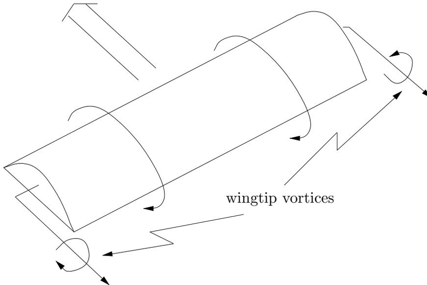
Figure 10.9. Lift from a wing of finite length.
