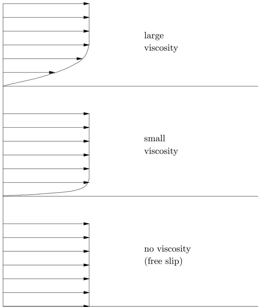
Figure 10.1. Illustration of flow parallel to a flat plate in the case of large viscosity, small viscosity, and no viscosity. The last case differs fundamentally from the other two in that no layer of vorticity exists at or just above the surface.
