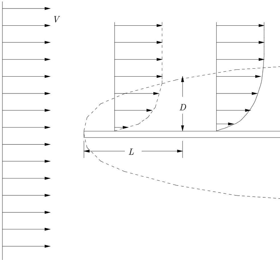
Figure 8.4. Initially uniform flow past a flat plate aligned with the flow. A boundary layer forms next to the plate, in which the fluid velocity is reduced from its initial value. The boundary layer thickens with increasing distance behind the leading edge of the plate.
