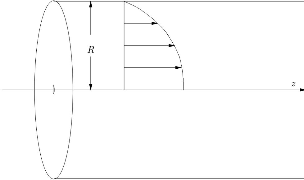
Figure 9.2. Sketch of laminar flow through a pipe of radius  $R$ .
