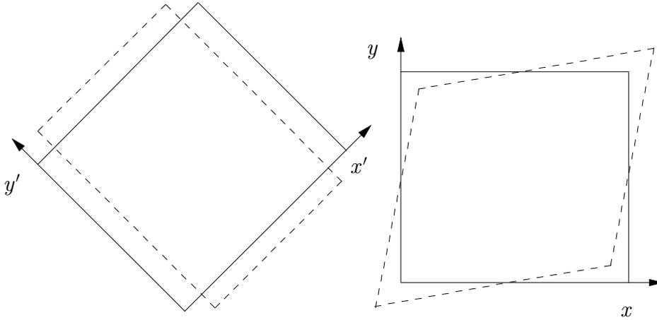
Figure 4.3. Effect of strain on two squares rotated  $45^\circ$  relative to each other.
