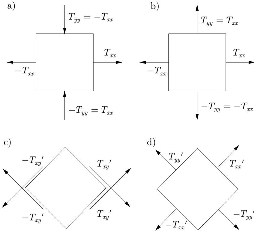
Figure 2.7. Tractions on edges of a square in two different cases, a)  $T_{yy} = -T_{xx}$ , and b)  $T_{yy} = T_{xx}$ , with  $T_{xy} = T_{yx} = 0$ . When the square is rotated by  $45^\circ$ , c) and d) show the transformed tractions.
