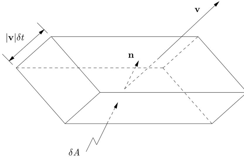
Figure 3.2. Sketch of flow through a surface element  $\delta A$  with unit normal  $\mathbf{n}$ . The volume of the parallelepiped,  $\delta A \mathbf{n} \cdot \mathbf{v} \delta t$ , equals the volume of fluid passing through the surface element in time  $\delta t$ . The fluid velocity is  $\mathbf{v}$ .
