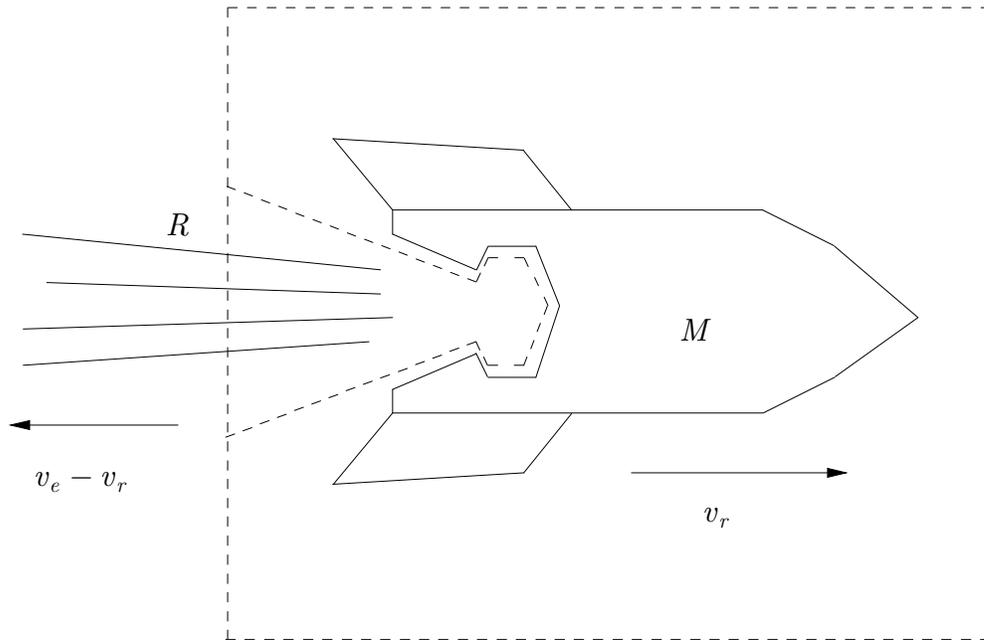
Figure 3.4. Sketch of a rocket moving to the right with speed  $v_r$ . The rocket has mass  $M$ , and is losing mass at the rate  $R$  via an exhaust with exhaust velocity  $v_e$ .
