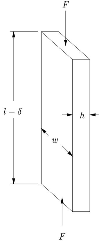
Figure 7.5. Definition sketch for buckling calculation.
