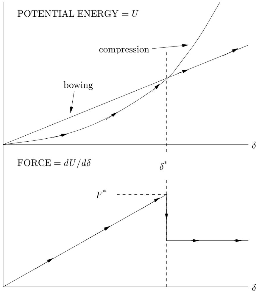
Figure 7.7. Potential energy of a beam shortened by an amount  $\delta$  under the influence of compressive forces on the ends, and the force required to maintain this reduction in length. Note that at the transition from compression to buckling at  $\delta = \delta^*$ , the required compressive force drops by a factor of two.
