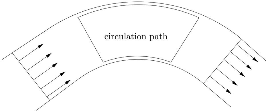
Figure 10.10. Water flowing irrotationally in a curved channel.
