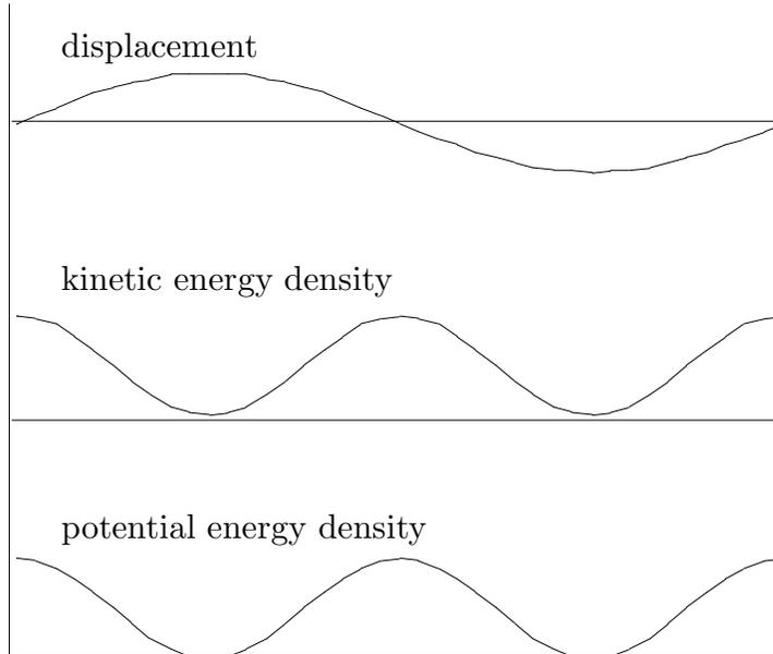
Figure 6.2. Relationship between wave displacement kinetic and potential energy densities in an elastic wave.
