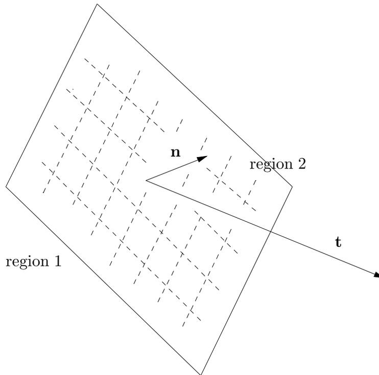
Figure 2.3. Illustration of the traction ( $\mathbf{t}$ ) and unit normal ( $\mathbf{n}$ ) vectors relative to a surface cutting a continuous medium. The traction is the force per unit area of region 2 acting on region 1.
