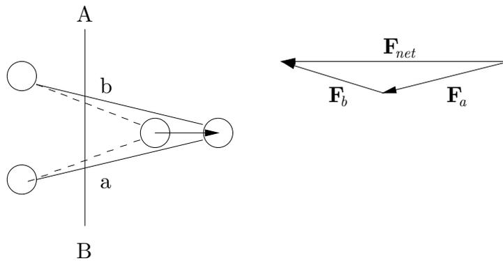
Figure 2.2. Relation between displacement and force on a molecule.
