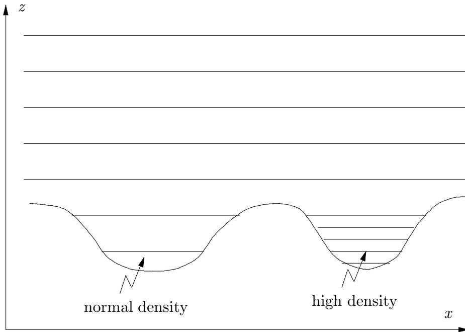
Figure 8.3. Contours of constant density of a fluid at rest in a container with an undulating bottom. Fluid parcels at the same level in “valleys” isolated from each other can have different densities. This cannot occur for parcels above the “ridgeline”.
