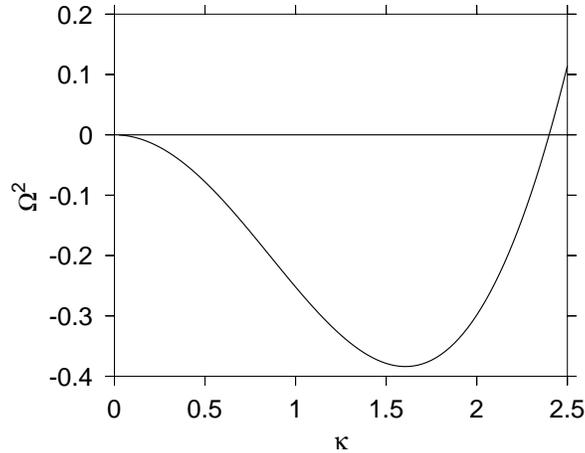
Figure 12.5: Plot of equation (12.69), dispersion relation for baroclinic instability. Instability occurs when  $\Omega^2 < 0$ , which is confined to the approximate range  $0 < \kappa < 2.4$ . The maximum growth rate occurs near  $\kappa = 1.6$ , at which point  $|\Omega| = 0.62$ . For  $\kappa > 2.4$ , a steady propagating wave occurs.
