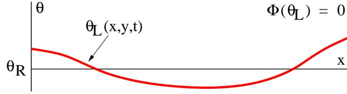
Figure 12.2: Illustration of lower boundary surface  $\theta_L(x, y, t)$  where the geopotential is assumed to equal zero.
