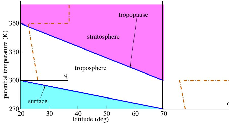
Figure 12.1: Schematic of north-south structure of atmosphere in middle latitudes. The surface tilts down to the north in isentropic coordinates, as does the tropopause. The dash-dotted lines show profiles of ambient potential vorticity as a function of potential temperature at two latitudes.
