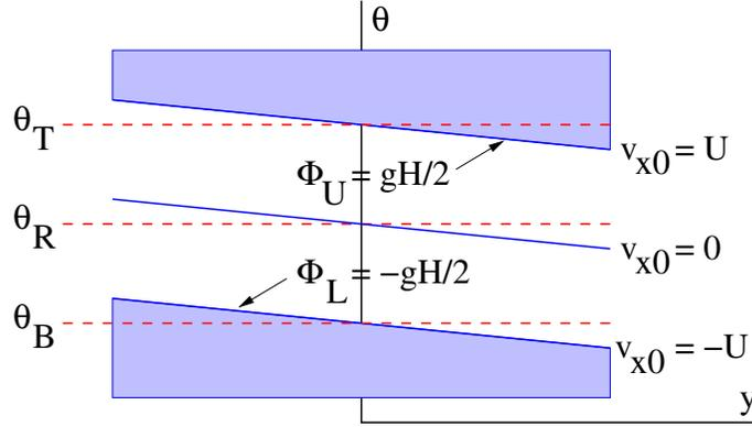
Figure 12.4: Idealized baroclinic environment in the Boussinesq approximation. The shaded areas indicate the bounding surfaces. The tilt downward with  $y$  of the geopotential surfaces in isentropic coordinates is geostrophically related to the increase in the  $x$  component of the ambient wind with height.
