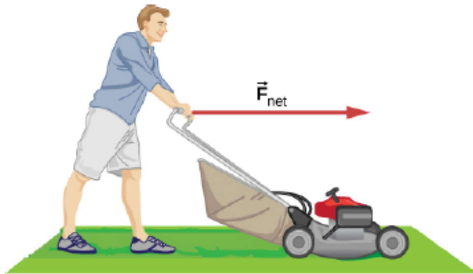
Figure 5.12 (a) The net force on a lawnmower is 51 N to the right. At what rate does the lawnmower accelerate to the right? (b) The free-body diagram for this problem is shown.
