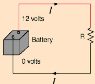
The electric current is the charge flowrate and it must be the same at any cross-section of the circuit. This is a general principle called the current law.
