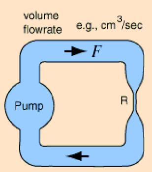
With continuous circulation around the pipe system, the volume flowrate must be the same at any cross-section of the pipe system.
